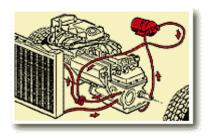
**REMCO'S Lube-Pump** lubricates and cools the Front Wheel Drive, Select rear Wheel Drive, Four-Wheel Drive, and All Wheel Drive vehicles while towing.
