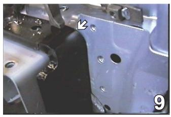
Cut the flat webbing on the top of the frame end. Do this to both sides of the vehicle.
