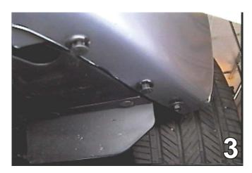
Remove the four metric bolts from the bottom edge of the front fascia with the 10MM socket and seven pushpins. Pull the fascia forward, set it and the pushpins aside to be reinstalled later.
