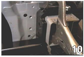
10. Set the baseplate in place on the frame ends as shown. Slide it as far back as possible and clamp it with the large vise grips. Do this to both sides of the vehicle.
